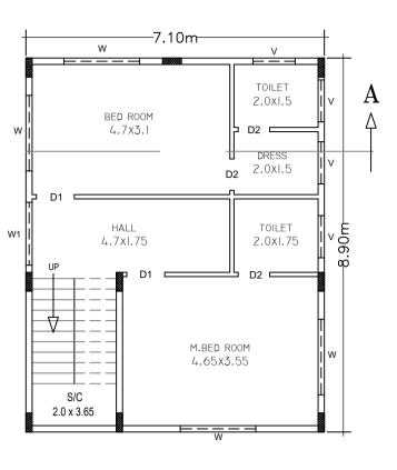
SECOND FLOOR PLAN (Proposed) (SCALE 1:100)
